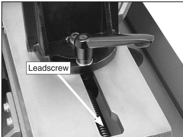
Figure 51. Typical vise leadscrew lubrication area.
